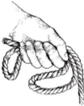
Correct method of holding the lead line
