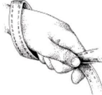
Incorrect method of holding the lead line
